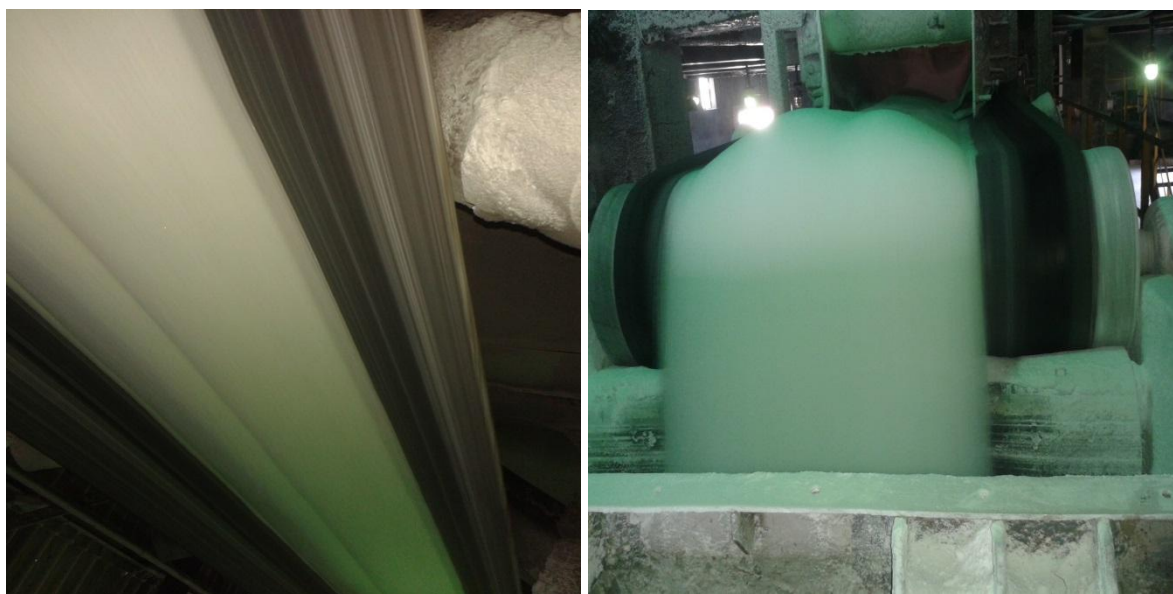
Fig. 5(Neem Coated urea on belt conveyor)
